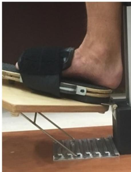
**Figure 1D:** Image of the syndhoo device from the side with the foot placed on the rotating board in 20 degrees of dorsiflexion.
