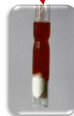
Figure III.10 - Qualitative demonstration of a simulated vessel occlusion thanks to the shape-memory PCL-CAN foam.
