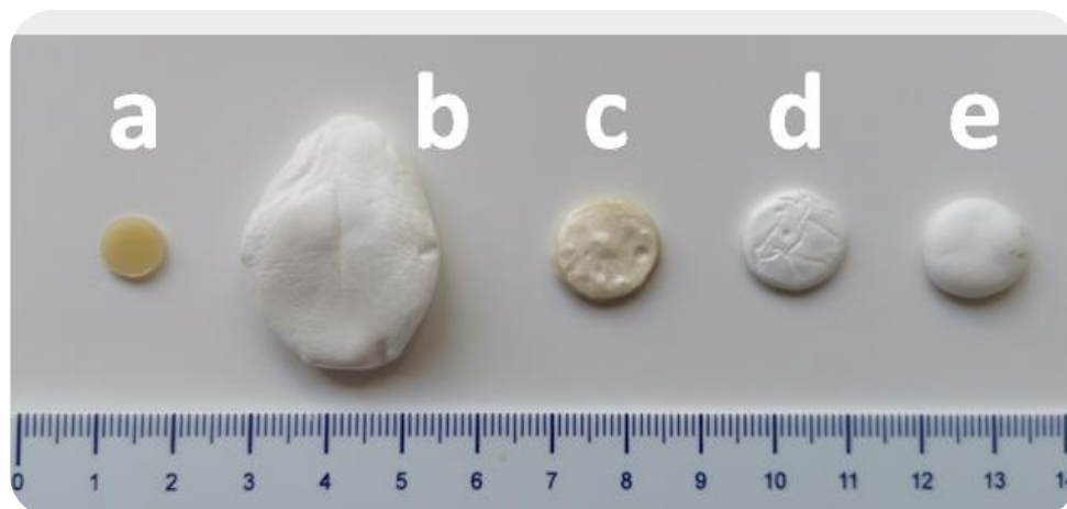
Figure III.2 - (a) PCL-CAN disk before foaming, and foams of (b) PCL-CAN disk cured at 105 °C for 1 hour, (c) PCL-CAN disk cured at 65 °C for 72hours, (d) PCL-PU network, (e) linear high molar mass PCL.
