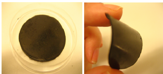
Fig. 4: Buckypapers made of MWNT dispersed in water (without surfactant). Flexibility of these buckypapers is here demonstrated.
