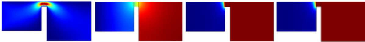
Figure 7: From left to right: the velocity field (0 – 0.0236 m/s), the electron concentration (0 – 2.297 \cdot 10^{-3} \text{ mol/m}^3 ), the O radicals concentrations (0 – 1 mol/m 3 ) and the CO concentration (0 – 1 mol/m 3 )
