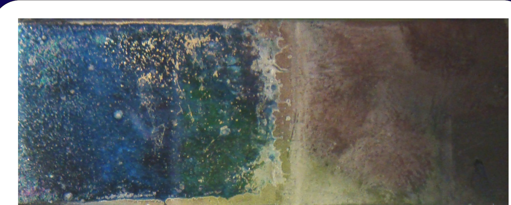
Figure 6: Chemochromic film turns in blue in presence of H 2 .
