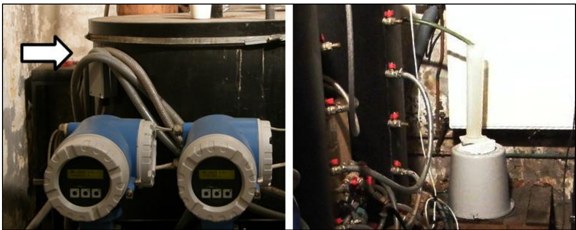
Figure 5-2 Flow meters adjustments and graduated cylinder used for measurement verification
