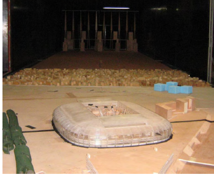
Figure 7. Model of the stadium in the wind tunnel.
