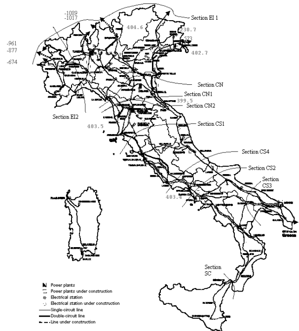
Fig. 7. One-line diagram of the 400-kV Italian system. Critical interfaces ( sections ) are highlighted. Reported numbers are OMASES VSA output
