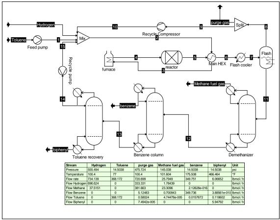
Figure 3 : HDA process (COFE software)
