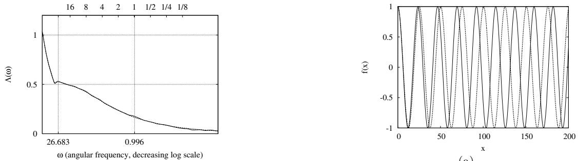
Fig. 8. The scale spectrum \Lambda of a realization of an AR(1) model Z with \alpha = 0.25 (solid lines) superimposed to a mean spectrum of the same AR(1) model (1000 realizations, dashed lines).
