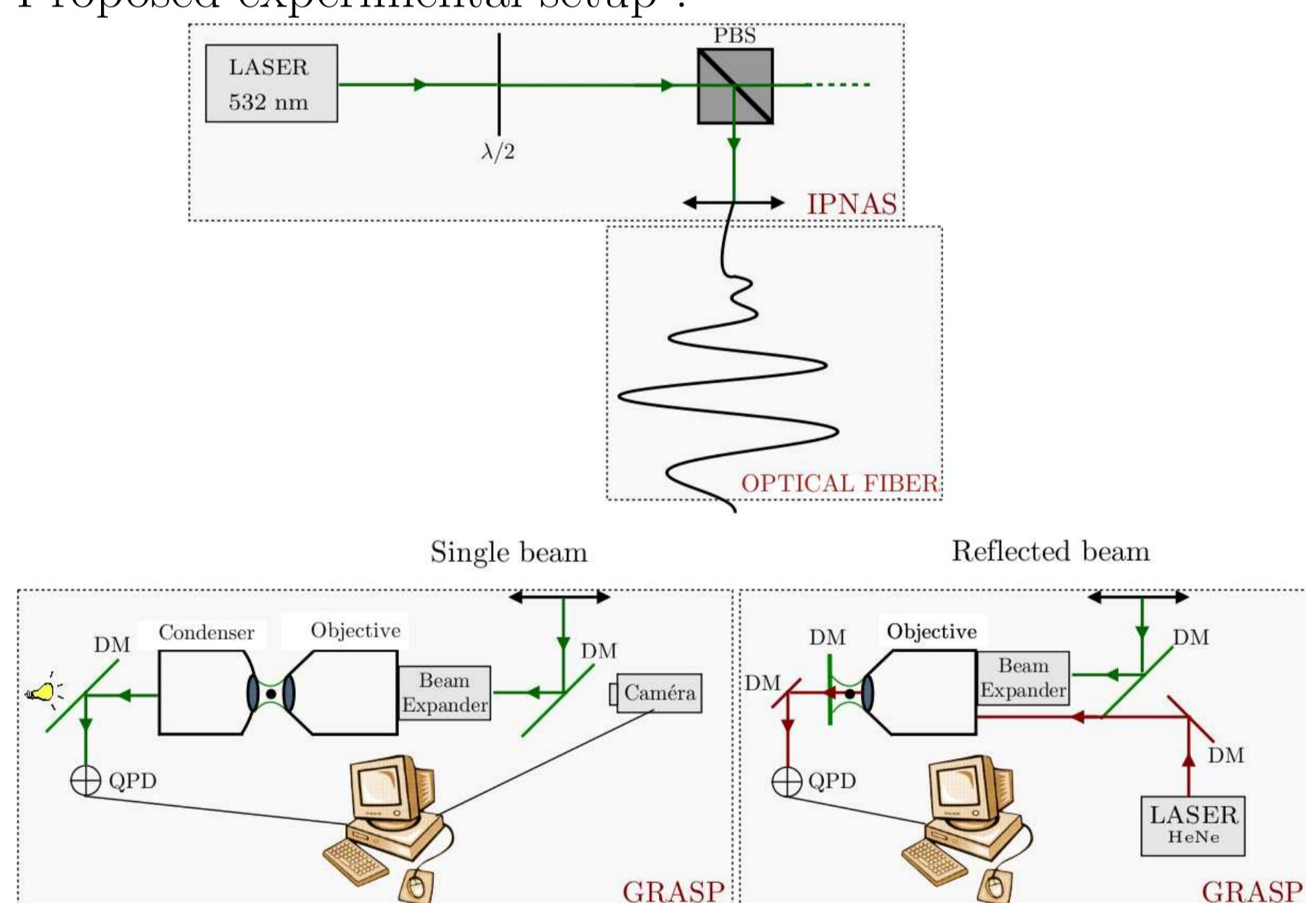
**Laser :** High power ( $\sim 1\text{W}$ ), high pointing stability ( $\sim \pm 50\mu\text{rad}$ ), low power fluctuation (1-2%).
