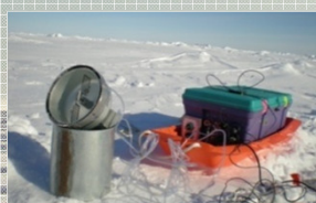
fig.1. – accumulation chamber for air-ice CO 2 fluxes measurements
