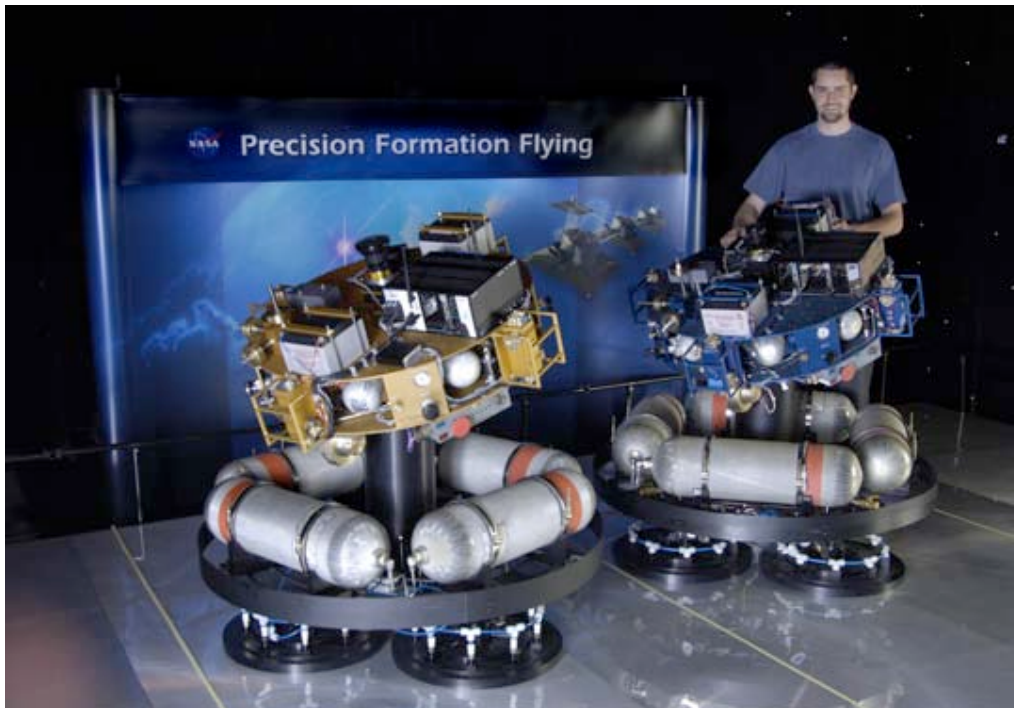
Figure 4-23. The Formation Control Testbed (FCT). Shown here are the two robots of the FCT. Each robot carries cannisters of compressed air that allow them to float off a polished metal floor. The floor is flat to within 2 one-thousandths of an inch and spans a much larger area than shown here. The robots serve as the hardware interface and testing ground for flight software developed for space applications in formation flying. (Courtesy Caltech/JPL/NASA)
