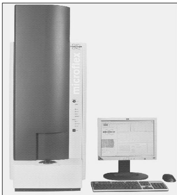
Figure 1. Microflex MALDI-TOF MS (Bruker Daltonics).
