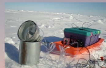
fig.1. – accumulation chamber for air-ice CO 2 fluxes measurements
