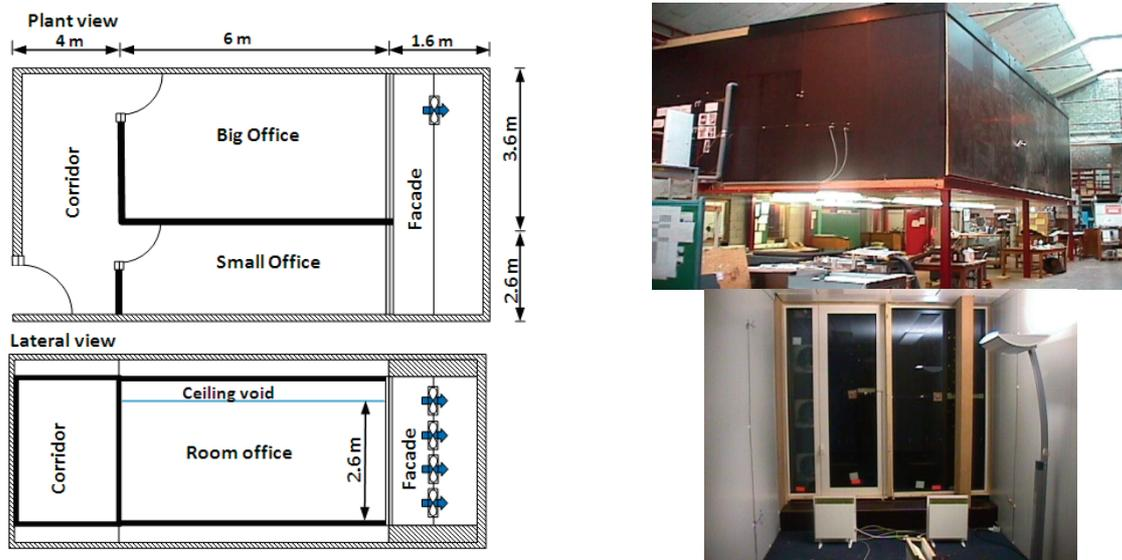
Figure 2 Climatic chamber: Plan and lateral views. External and internal views
