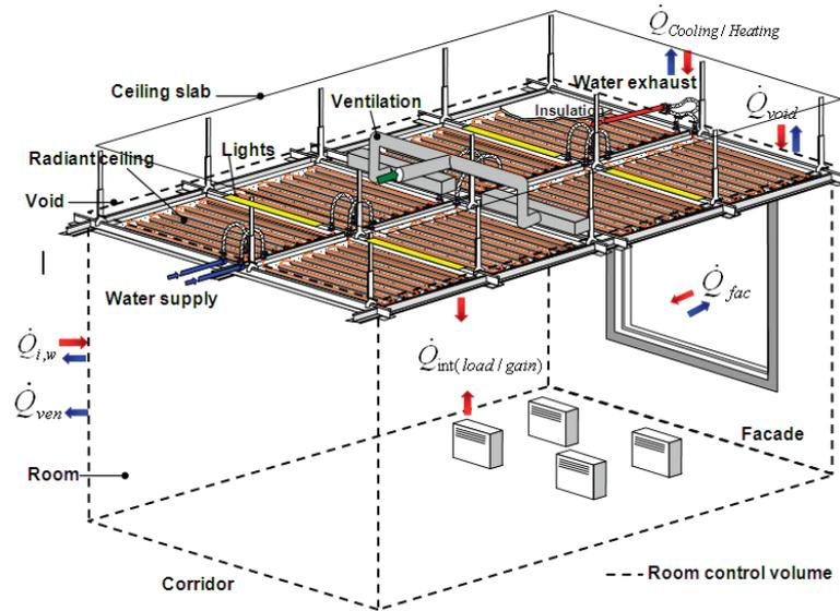
Figure 3: Control volume for the room global balance
