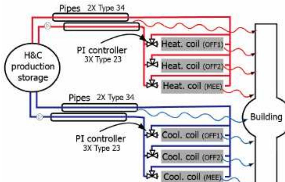
Pipes, pumps, control and fan coil units are modelled
