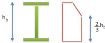
Figure 14_Simple temperature profile between the levels of top and bottom flanges
