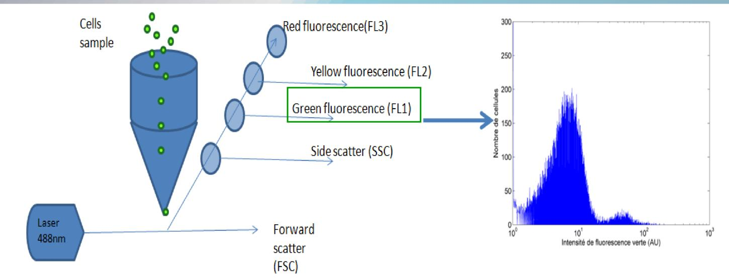
Flow cytometry allows the green fluorescence analysis at the single cell level:obtained results are frequency histograms of fluorescence-intensity in the microbial population. So, it is possible to link the GFP content among the microbial population with the bioreactor heterogeneity (stress condition)
