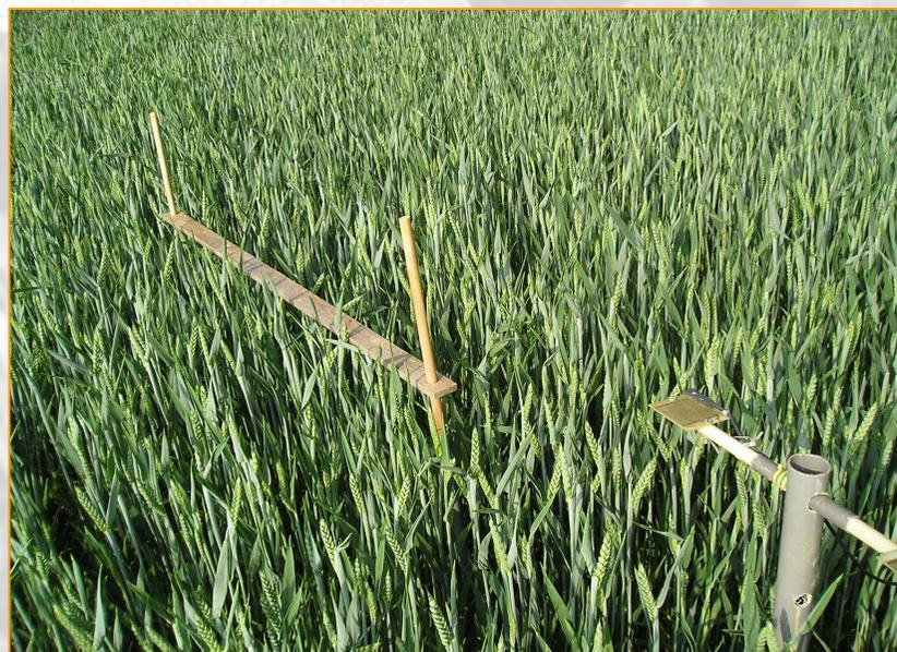
**Collect the amount of dew water that deposited on rigid epoxy plates placed next to each sensors.**
