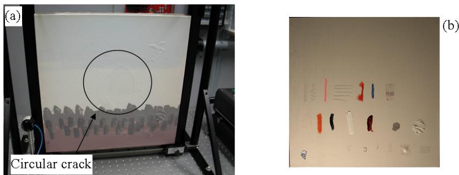
Figure 2. (a) Representative sample of painting on textile canvas. A circular crack is barely visible inside the red circle. (b) Artificial defects/inclusions present between the canvas and the paint layer.
