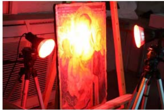
Figure 2: Example of a panel painting examined with non-contact, non-destructive full field interferometry
