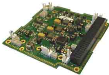
Figure 1.6 – Main EPS engineering model
