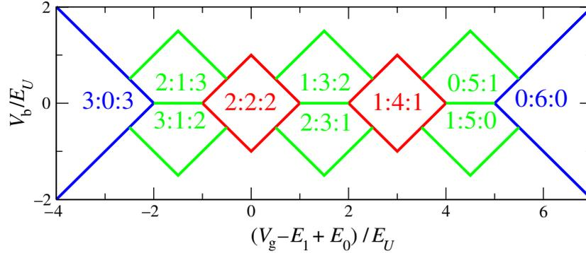
**Figure 5.** Structure of the interaction-blockade diamonds that result from a simple Bose–Hubbard-type model. Plotted are the predicted transition lines for single-particle transfer between adjacent wells according to equations (14) and (15), assuming the presence of six particles in a triple-well potential with equal on-site interaction energies. The agreement with figure 4 is rather good, taking into account the approximate value  $E_U \simeq 0.268V_0$  (4) for the interaction energy.
