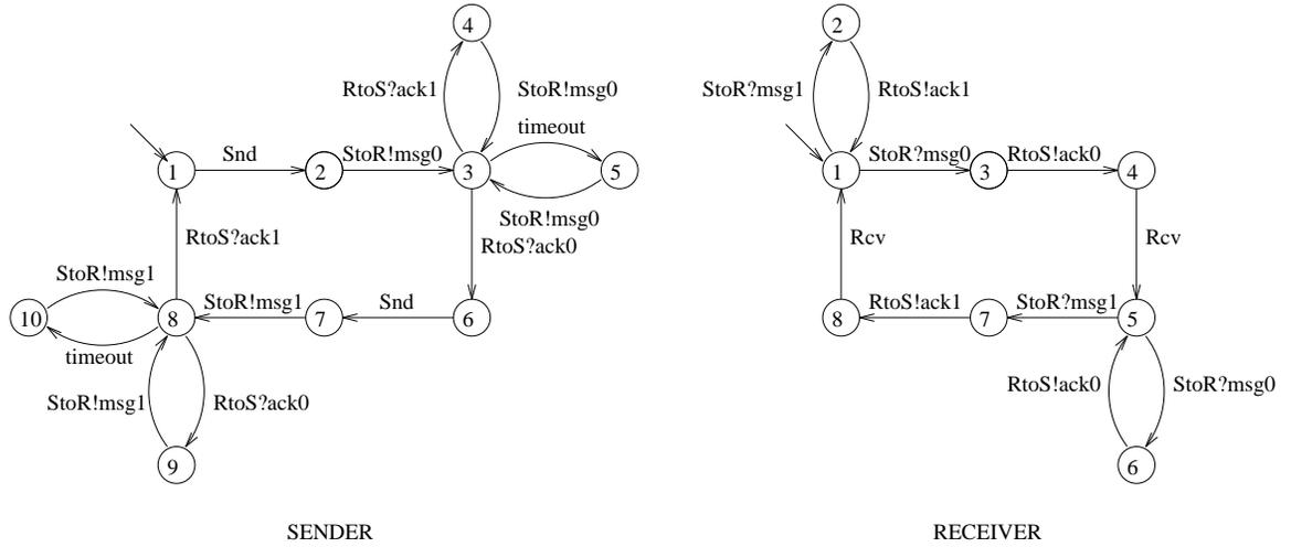
Figure 1. Alternating-Bit Protocol
