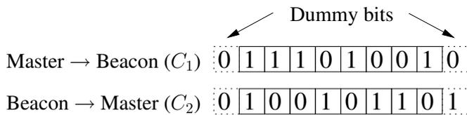
Figure 5. Codes used for the communication between the master and the beacon ( $C_1$ ) and between the beacon and the master ( $C_2$ ). The first and last bits surrounding the codes are the dummy bits.
