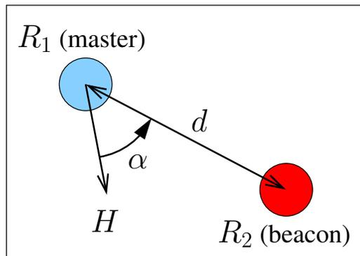
Figure 1. Upper view of the EUROBOT playing field with the two robots  $R_1$  and  $R_2$ . The purpose of our platform is to get unambiguous and reliable range measurements  $d$  from our robot  $R_1$  to the opponent robot  $R_2$ . This range measurement is to be combined with the angular position  $\alpha$  (from our robot heading  $H$ ) given by the system described in [8] to compute the full position of the opponent robot.
