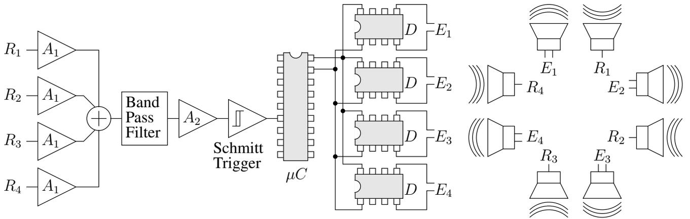
Figure 2. Bloc-diagram of the emitting and receiving part of the master or beacon.  $E_i$  are the ultrasonic emitters,  $D$  are the MAX232 drivers, and  $\mu C$  is the common microcontroller.  $R_i$  are the ultrasonic receivers,  $A_1$  are the pre-amplifiers and  $A_2$  is the second amplifier.
