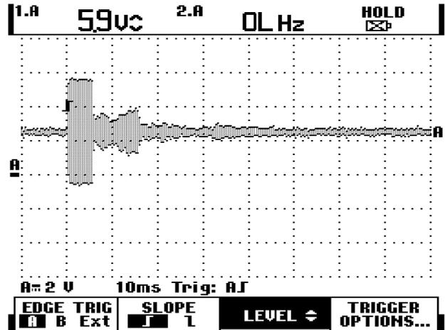
Figure 4. Falling time of an ultrasonic emitter/receiver pair after a 6 [ms] burst at the central frequency  $f_c = 32.8 [kHz]$ . The receiver continues to oscillate for a long time after the pulse has stopped. The falling time is about  $t_f = 50 [ms]$ .
