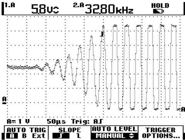
Figure 3. Rising time of an ultrasonic emitter/receiver pair for a step at the central frequency  $f_c = 32.8 [kHz]$ . The rising time is about  $t_r = 150 [\mu s]$ .
