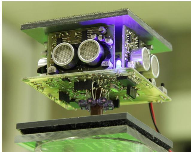
Figure 6. Picture of the ultrasonic beacon onto the opponent robot. One can see the ultrasonic transducers arranged in four pairs of emitters and receivers at the upper side. Below are the IR emitting diodes of the system described in [8].
