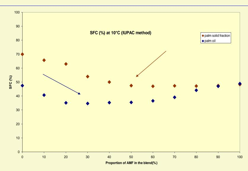
Under dynamic conditions, a minimum is observed (eutectic interaction) within the SFC-lines as a function of composition, for all the blends.
