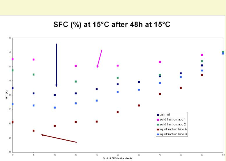
After the tempering procedure, the minimum of SFC is observed for higher HLERO content in the case of blends involving « solid fractions » and for lower HLERO content in the case of blends involving « liquid fractions » compared to blend made of full palm oil.
