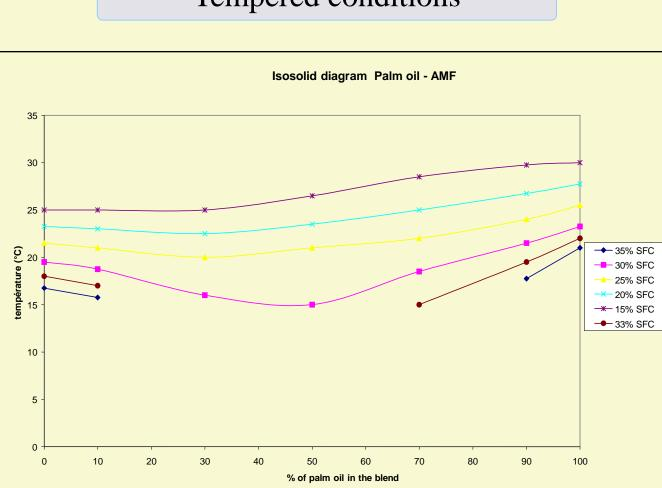
After a tempering procedure, Isosolid lines corresponding to lower SFC (upper lines) increase with increasing content of palm oil in the blend (specially palm oil content > 30%). Isosolid lines corresponding to higher SFC (lower lines) don't follow that behavior: a minimum is observed for the 50-50% composition (eutectic interaction)
