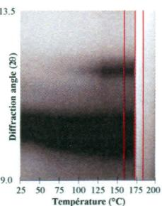
Temperature-Resolved WAXS of semi-crystalline inulin stored one week at 94% RH (water content = 20.8 g water / 100 g dry inulin). Vertical lines correspond to the onset, midpoint and endset temperature of the MDSC endothermic peak centered at 170°C.
