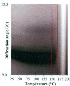
Temperature-Resolved WAXS of amorphous inulin stored one week at 94% RH (water content = 18.9 g water / 100 g dry inulin). Vertical lines correspond to the onset, midpoint and endset temperature of the MDSC endothermic peak.
