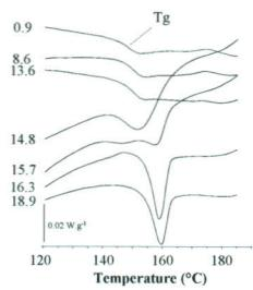
Up to 13.6 g water / 100 g dry inulin, amorphous inulin only presented a glass transition at around 150°C. Although the samples at 14.8 and 15.7 g water / 100 g dry inulin were still amorphous, their thermal properties were different from those containing up to 13.6 g water / 100 g dry inulin. Above 16.3 g water / 100 g dry inulin, an endothermic peak was present around the glass transition temperature.
