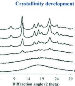
The samples were considered completely amorphous up to a water content of 15.7 g water / 100 g dry inulin (crystallinity index = 0%); while crystallization occurred between 15.7 and 16.3 g water / 100 g dry inulin. The crystallinity indexes increased up to 92-93% at 18.8 g water / 100 g dry inulin.
