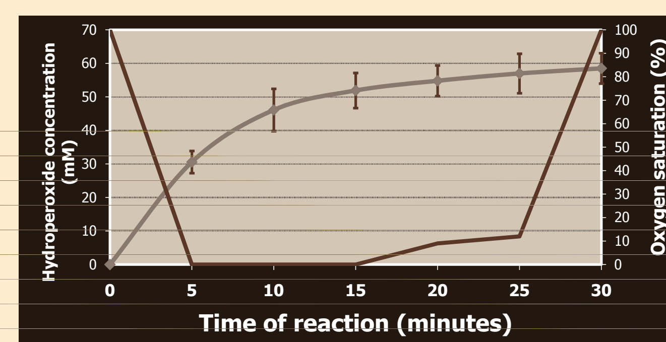
Fig. 1 : Biotransformation of 100mM linolenic acids solution into hydroperoxide by 13-Lipoxygenase. Grey line represents the hydroperoxide concentration during reaction, and brown line the oxygen level in bioreactor.
