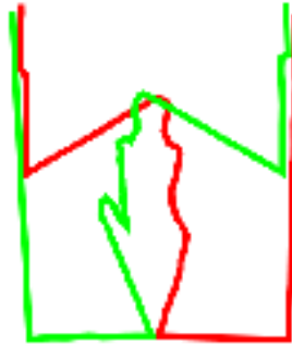
Figure 3. Construction of a curve per sensor that corresponds to the closest visible points. The signal captured by the left (right) sensor is displayed in green (red).
