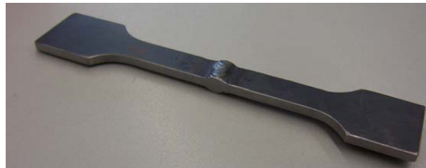
Figure 4-50 : Butt welded joints used for the tests on welds under natural fire
