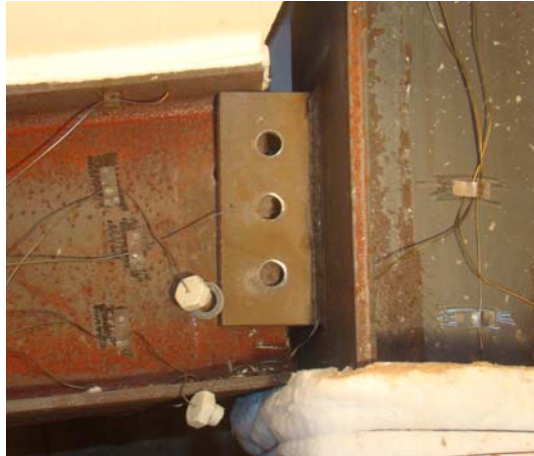
Figure 6-5 : Fin plate connection after failure of the connection
