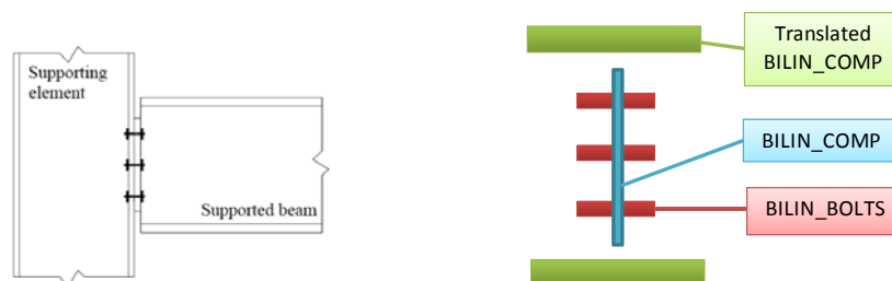
Figure 6-23 : Header plate connections (left) and Bilinear Fibre Model (right)
