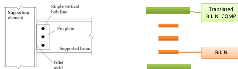
Figure 6-19 : Fin plate connection (left) and Bilinear Fibre Model (right)
