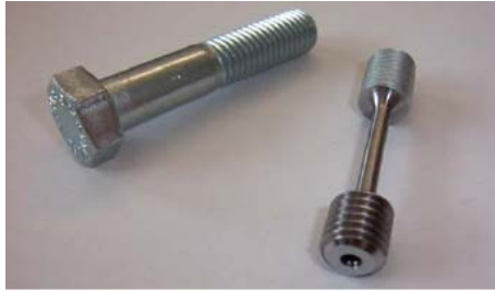
Figure 4-6 : Intact bolt and machined specimens tested to characterise the bolt material
