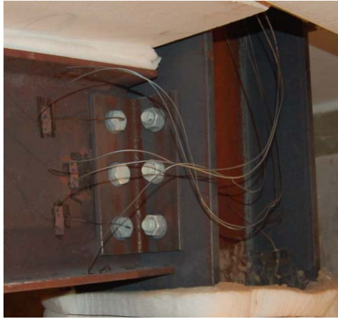
Figure 6-7 : Double web cleats connection after the test
