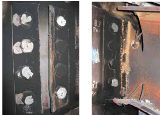
Figure 6-48 : Failures of the two joints by header plate and beam web tearing [Santiago, 2008b]
