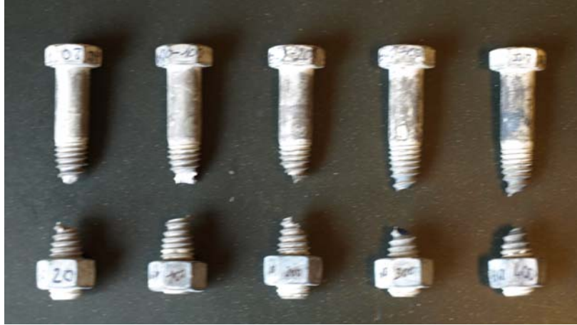
Figure 4-7 : Bolts tested in tension after natural fire at different T_f temperatures after reaching T_u = 600^\circ\text{C}
