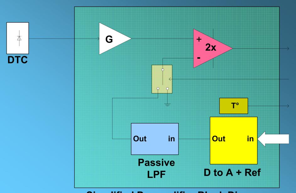
**Simplified Preamplifier Block Diagram**
