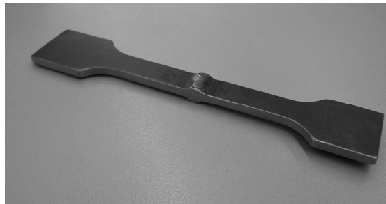
Figure 10. Specimen submitted to transversal tensile forces during weld tests
