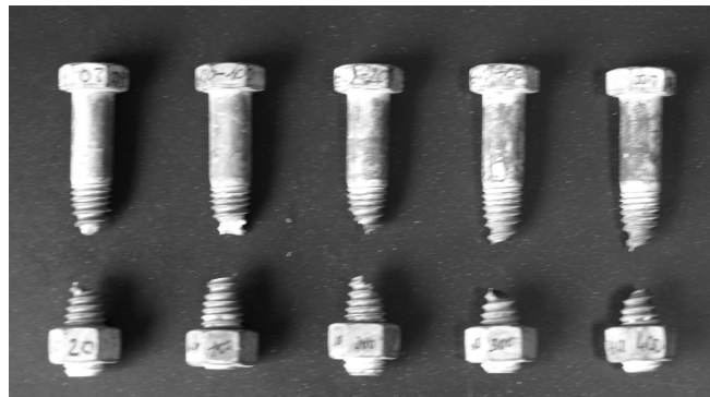
Figure 4. Bolts tested in tension ( T_u = 600^\circ\text{C} )
