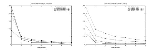
**Fig. 4.** Average bandwidth (in Kbps) consumed by AYA over all the links in random 60 nodes network. (leftmost) AYA traffic generated by one average active node, (rightmost) traffic generated by all the active nodes together
