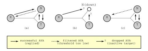
**Fig. 3.** A problematic scenario if down neighbours are not re-scanned periodically: (a) N is initially discovered by X which has a high threshold but X can't be discovered by N because it's out of its scope, (b) when N crashes, both X and Y notice it after their refresh AYA gets dropped, (c) after N recovered, only Y is able to detect it from N's boot-time scanning. X being out of scope, it believes N is still down
