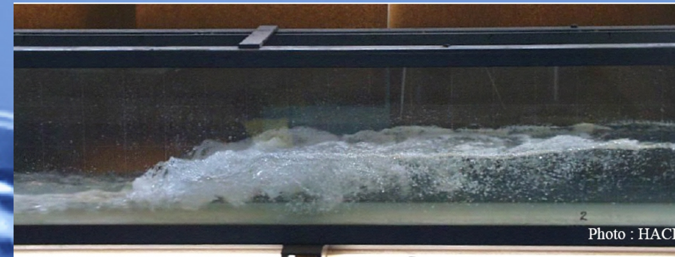
Aeration in a hydraulic jump. Source : HACH
