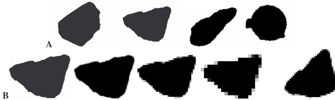
Fig. 2. A. Set of real particles (diamond, sand, rutile, glass bead) used for testing in addition to ellipses and disks. B. Sand particle sampled at 9000, 2300, 600, 140 pixels and rotated 30^\circ at 600.
