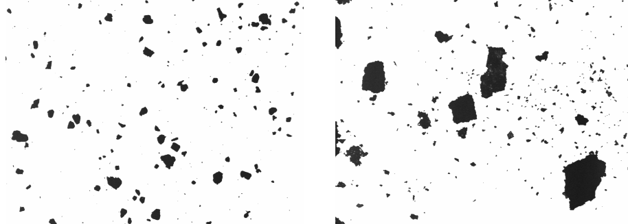
Fig. 1. Example of polydispersed granular materials (silica sand, dried food).
