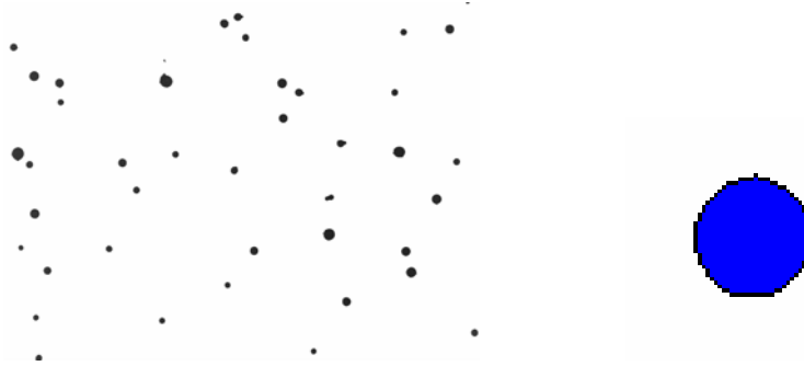
Fig. 3 Atomized particles imaged with a 1 MPixels video camera using a superzoom objective. Individual thumbnail image of a 15 µm particle as obtained from grey level thresholding.
