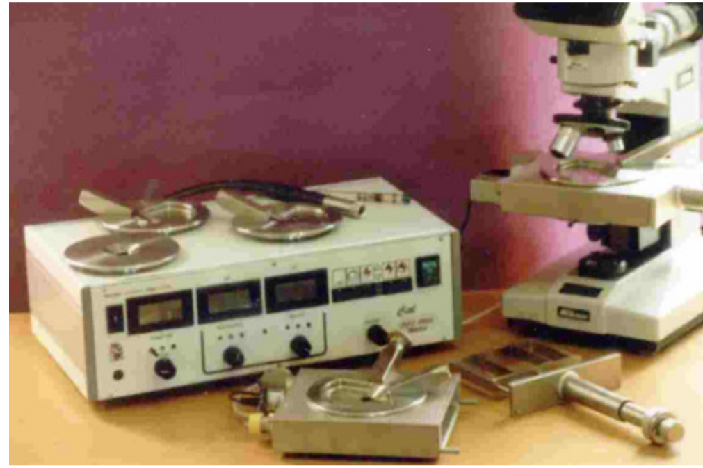
The Cold Cathode CL 8200 MK4 with various sample stages and gun geometries (doc. CITL)
