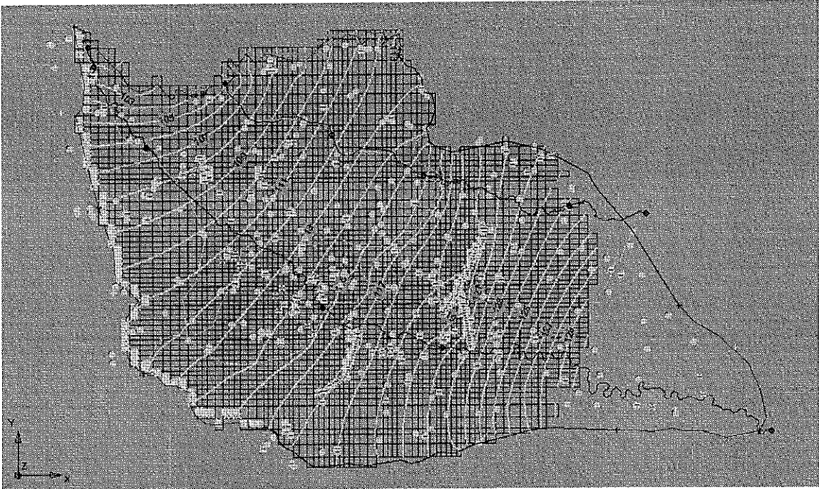
Figure 5. The regional groundwater flow model of the deep Szamos/Somes alluvial transboundary aquifer.
