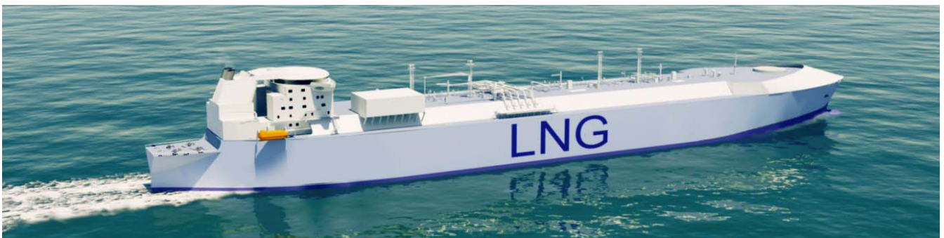
Figure 1. 220 000 m 3 LNG carrier studied by STX- France
