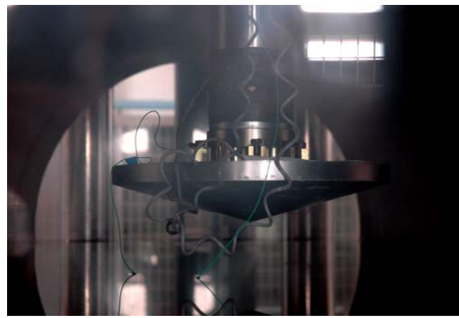
Figure 12: Experimental setup of the rigid cone
