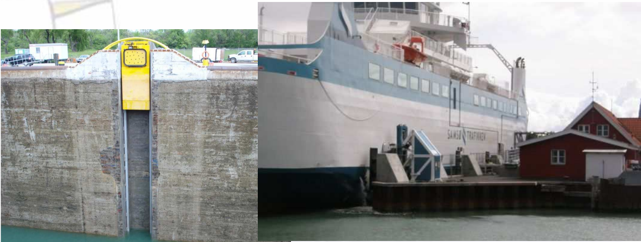
Magnetic Mooring System at KaiserLock (Cavotec Ltd)
