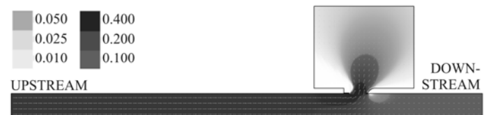
Figure 11 Unit discharge [m 2 /s] computed with FV model for test Q300-h50 with an elongated inflow channel
