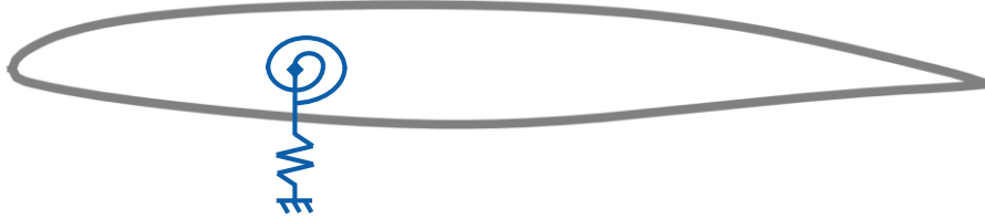
Figure 2: CAST 10-2 aerofoil with leaf and torsional springs.
