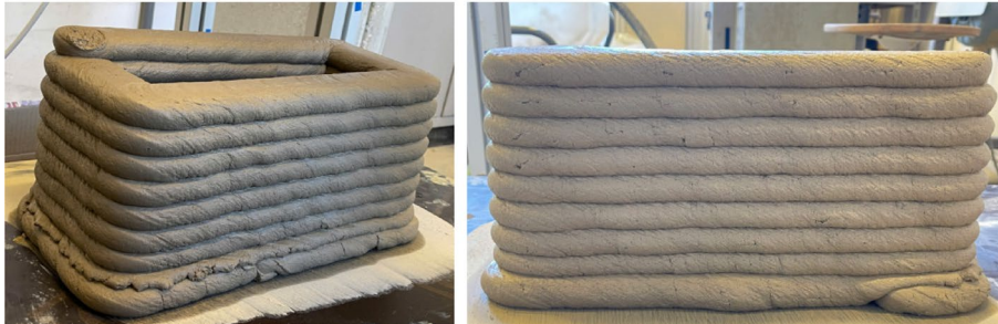
Fig. 15 The actual printing performance of (a) FIN 05 and (b) FIN 10
