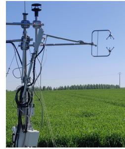
Figure 1.2: Eddy covariance system with a 3D sonic anemometer and a closed-path IRGA (BE-Lon).
