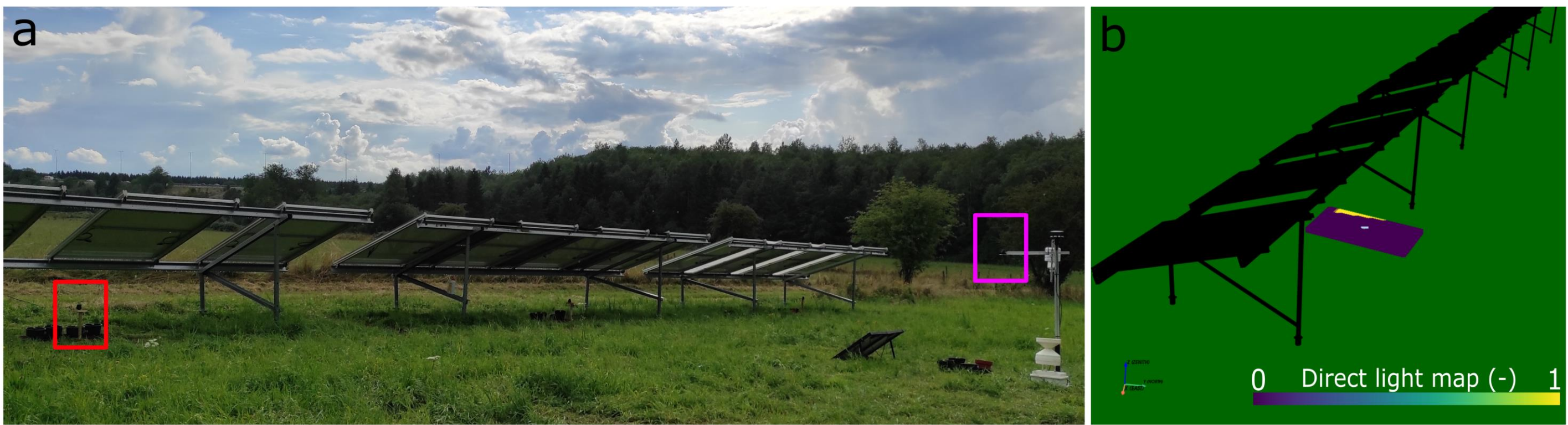
Fig. 1: Siguesol agrivoltaic prototype and experimental set up with full sun condition pyranometer in purple and agrivoltaic pyranometer in red (a) and experimental set up reproduced in PASE (b)
