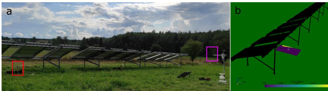
Figure 1. SigueSol agrivoltaic prototype and experimental set up with full sun condition pyranometer in purple and agrivoltaic pyranometer in red (a) and experimental set up reproduced in PASE (b).
