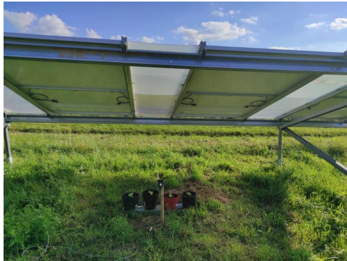
Figure 2. Picture of a real-world test lead in the field. Irradiance at ground level is smoothed by lenticular diffusers placed between solar modules.
