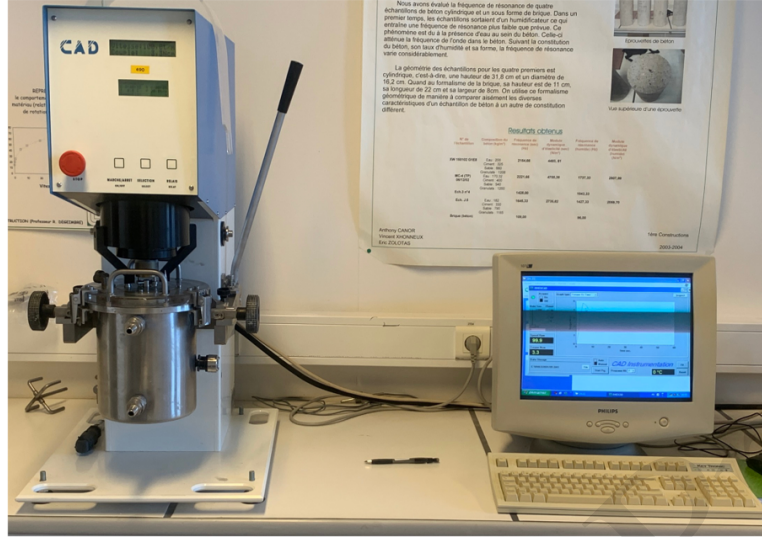
Figure 5. RheoCAD rotational rheometer used for the measurement of yield stress and viscosity
