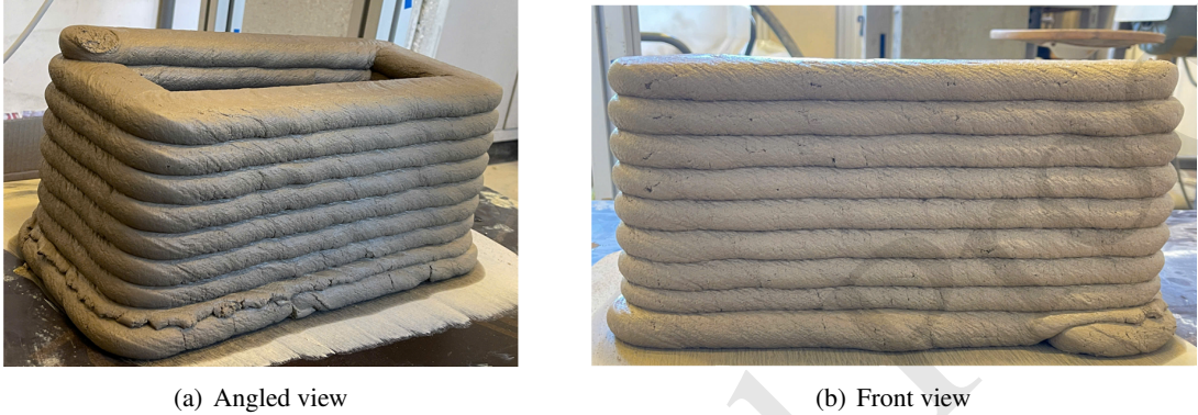
Figure 4. Hollow rectangular specimen of mix FIN 10 printed with the actual 3D printer
